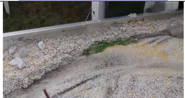
G5-12 EmRiver Introduction: erosion and deposition in a self-forming model river channel
