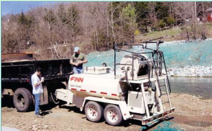
A hydroseeder is used to sow grass seed in riparian areas.
