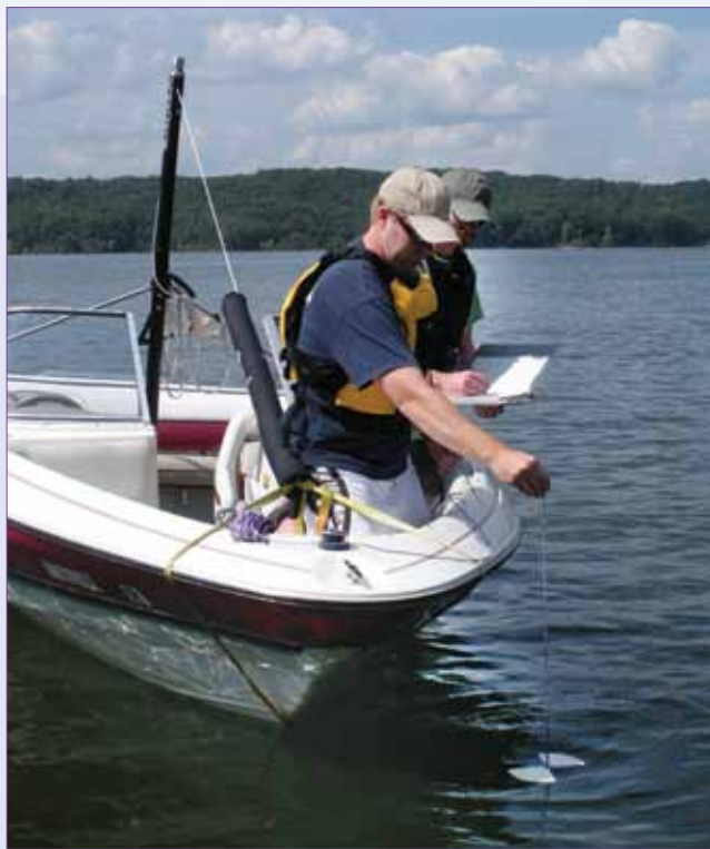
Citizen scientists use a Secchi disk, the black and white object at the bottom right of the photo, to measure water transparency.
