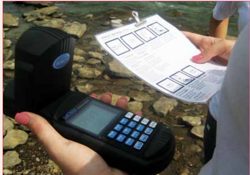
A member of the team conducts a nitrate test using a colorimeter.
